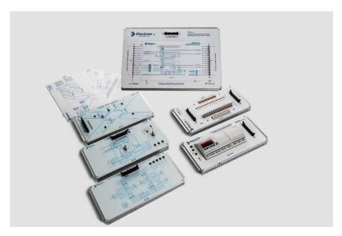
The laboratory is conceived to give the student a clear overview of the concepts involved in industrial automation. It includes a PLC automation trainer complete with a comprehensive series of industrial process simulation modules. A Pneumatic and electro pneumatic trainer, with a comprehensive set of typical components used in pneumatic control applications. The components are mounted on modules that can be installed on a panel frame or a bench for teacher demonstration and student use.
